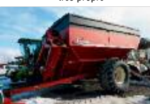
Grain Cart Parker 938 (2011), 950 minots, vis 17", balance, toile, clapet hydraulique, pneu 900/60-32
