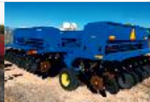
Semoir Landoll 5530, 30 pi, no-till, pneumatique pression, 2011
