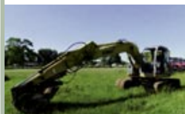
Excavatrice Kobelco 135, 13.5 tonnes
