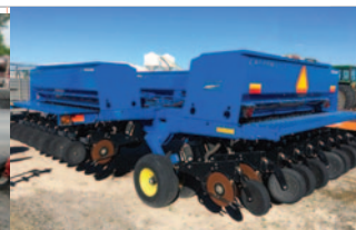
Semoir Landoll 5530, 30 pi, no-till, pneumatique pression, 2011
