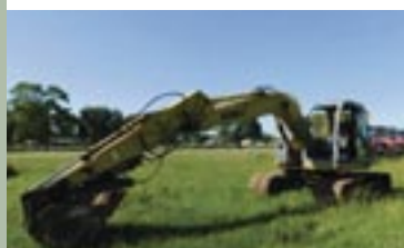
Excavatrice Kobelco 135, 13.5 tonnes
