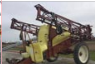
Arroseuse Hardi NP1100, 90 pi, 1100 gal., single jet, 5 sections, 320/90R46, suspension
