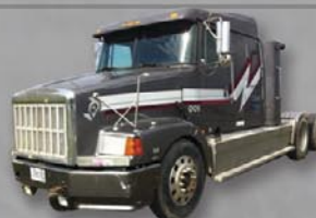
Camion Volvo VE D-12-425vt, transmission v11414, pompe huile
