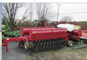
Semoir Sunflower 9434, 40 pi aux 7.5 po, engrais liquide, no-till
