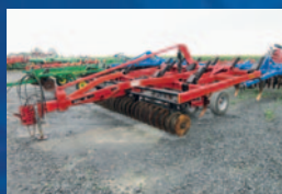
Chisel Case 6650, 11 pattes, disques droits, tandem
