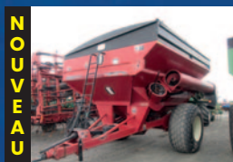
Grain Cart Brent 782, toile, balance isobus, 30.5-32 diamond, clapet rotatif
