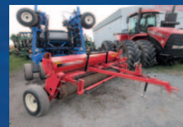
Semoir Brillion SS12, 2 compartiments, peigne, relevage hydraulique
