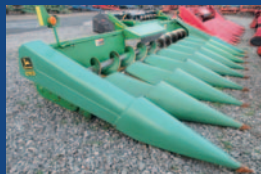
Nez à maïs John Deere 893, 8 rangs, deck plate ajustable hydraulique, single point, PTO
