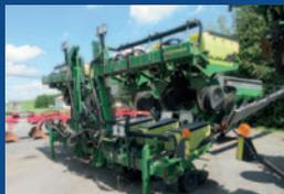
Planteur John Deere 1720, 12 rangs, stackfold, MaxEmerge XP, pression springs HD, kit engrais liquide Yetter, boîtes 3 bu, plaques Precision Planting, Vacuum, popu. hydr., ISOBus
