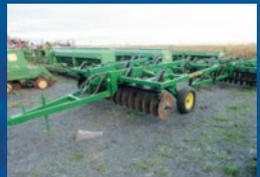
Chisel John Deere 714, 9 pattes, disques droits, relevage hydraulique, pointes neuve
