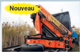
Grue Palfinger PK 9501 , 2008, 5 sections hydrauliques
