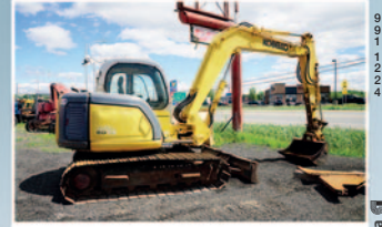
Excavatrice Kobelco 80CS , gratte avant, attache rapide, 1 godet
