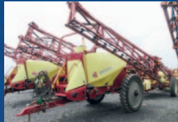
Arroseuse Hardi Navigator 4000, 2012, 100 pi, 6 sections, isoBUS John Deere, pompe hydraulique, jet triple
