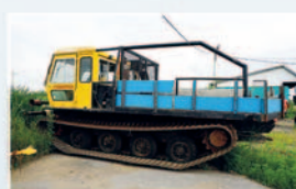
Chenille Bombardier Go-Tract GT-2000 WT , moteur diesel Cummins 8.3 l, transmission Spicer
