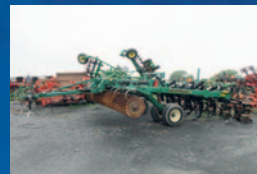
Chisel Great Plains TC5113, 13 pattes chisel, disques turbo ajustables hydrauliques, rouleau chopper arrière
