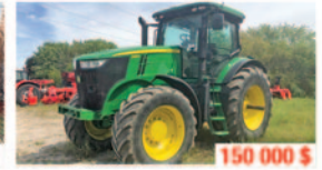
JD 7215R , 2014, 215 HP, 3400 h, transm. IVT, 40 km/h, susp. avant, 4 s.h., pneus 710/70R42 et 540/65R34
