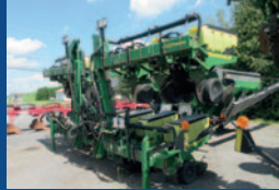
Planteur John Deere 1720, 12 rangs, stakfold, MaxEmerge XP, pression springs HD, kit engrais liquide Yetter, boîtes 3 bu, plaques Precision Planting, Vacuum, popu. hydr., ISOBus
