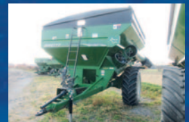
Grain Cart Brent 782, toile, pneus Continental 680/85R32, chute rotative hydraulique
