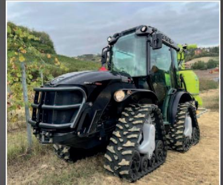
The Mach 4 R articulated and oscillating tractor (ACTIO), with a reversible driver's cab, is mounted on four tracks for better traction and less compaction.
