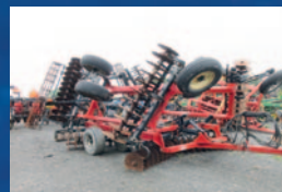
Herse Turbo Case True Tandem 330, 25 pi, rock flex, gros shaft, rouleau de finition
