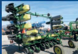
Planter John Deere 1710, 16 rangs, 22 po, 3 points, wheel assists, marqueurs, Track-250, 3 bu, tasse-résidus, vacuum, drive hydraulique
