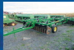
Chisel John Deere 714, 9 pattes, disques droits, relevage hydraulique, pointes neuves
