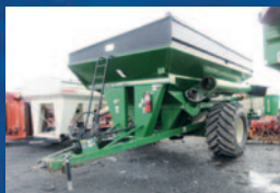
Grain Cart Unverferth 9250, toile, pneus 900/60R32, clapet hydraulique
