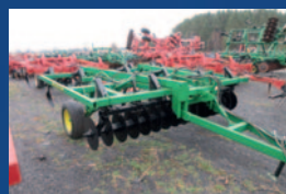
Chisel John Deere 714, 9 pattes, disques droits, ajustables hydrauliques
