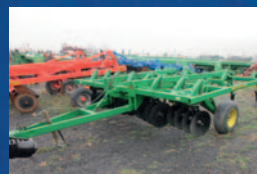
Chisel John Deere 712, 19 pattes, disques concaves, roues simple
