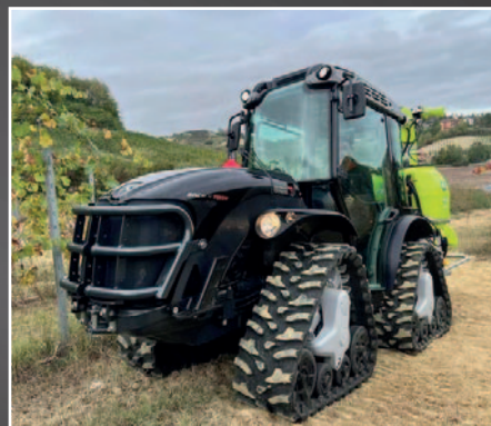
The Mach 4 R articulated and oscillating tractor (ACTIO), with a reversible driver's cab, is mounted on four tracks for better traction and less compaction.
