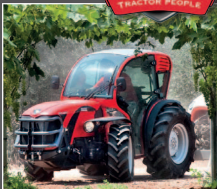
The low-profile tractors TGF 7800 S 4F with 71 hp and TGF 8900 R (shown) with 75 or 98 hp, with 16 x 16 transmission, travel up to 40 km/h.
