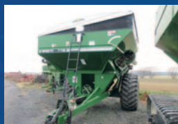
Grain Cart Brent 776, toile, balance Digistar EZ 2000, 30.5L-32
